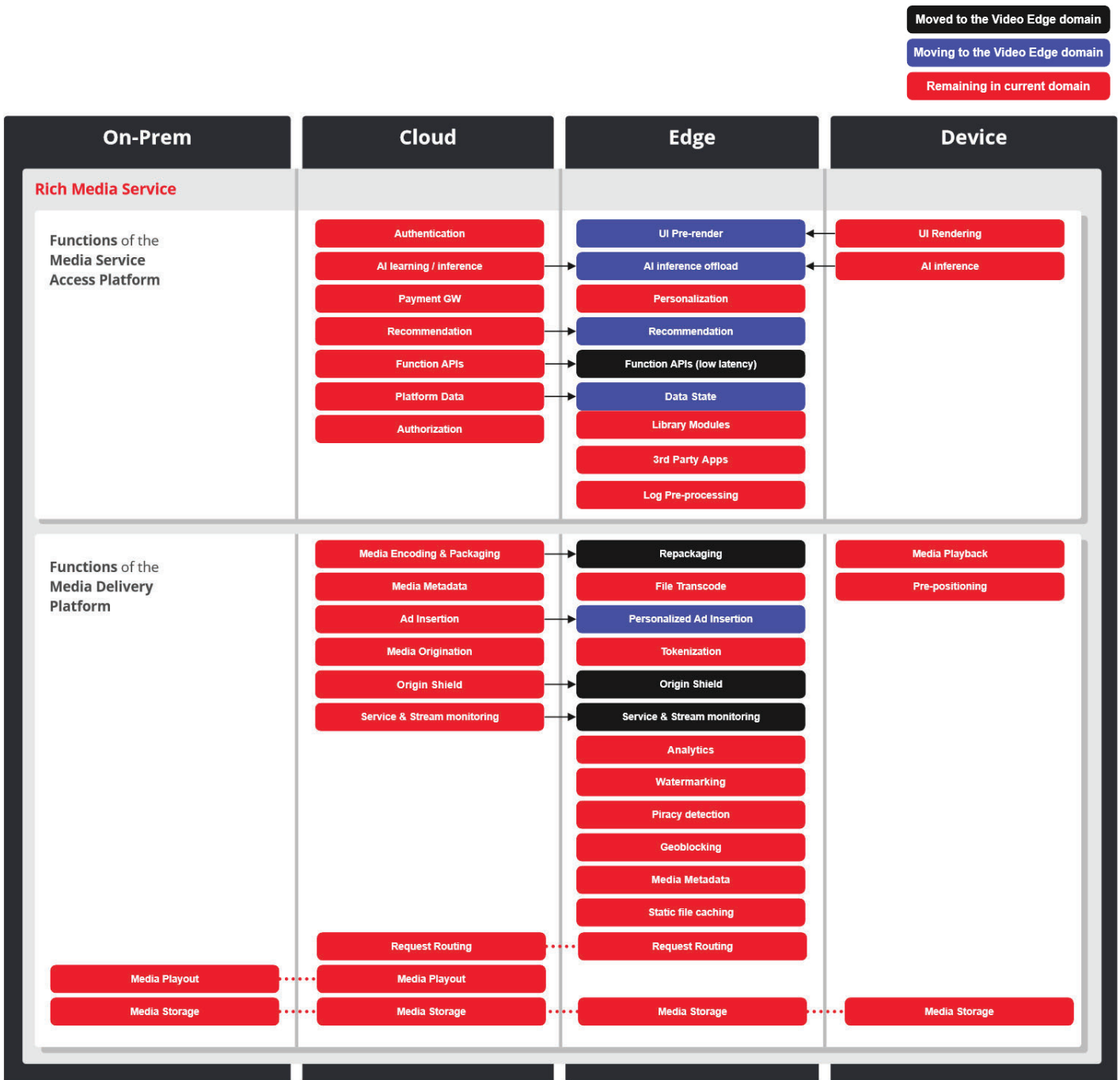
Figure 4: The Media Service functions already moved or currently moving into the Edge Computing domain.
