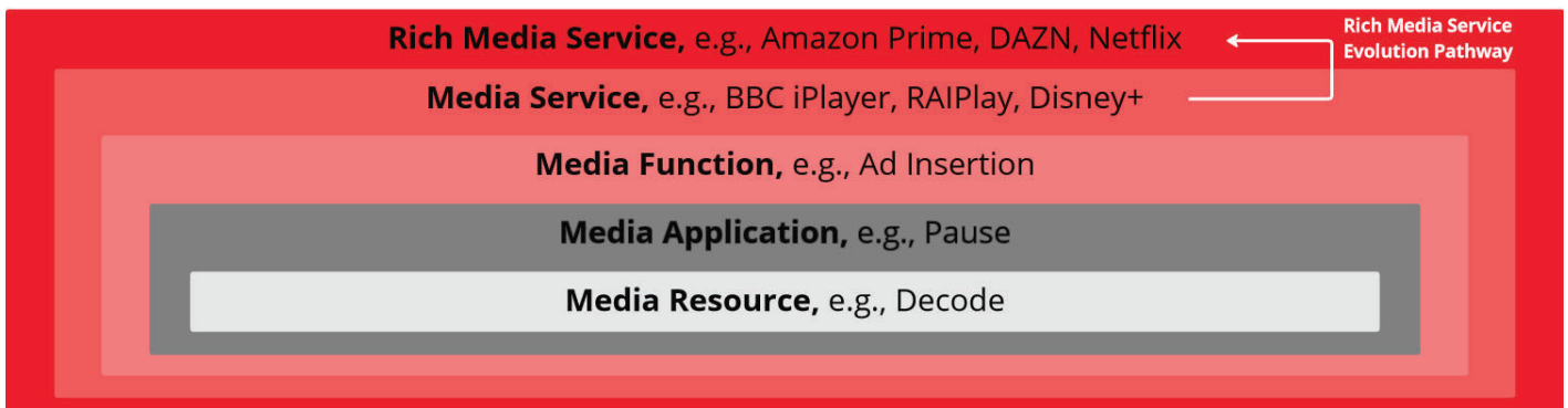
Figure 2: Rich Media Service Architecture Layers
